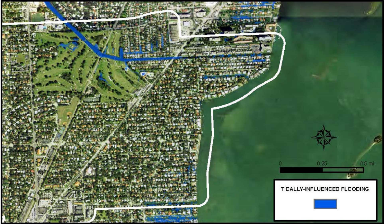
Figure 2 Tidal flooding prediction by Coastal Risk models during the highest tides for 2018.
